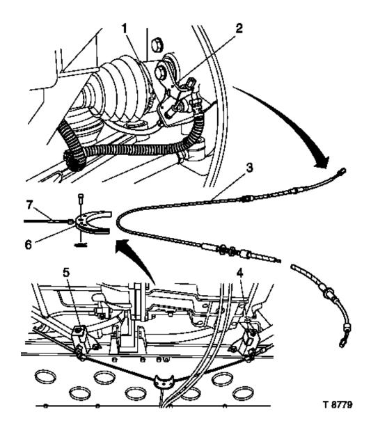
Lubricate components with suitable grease.
